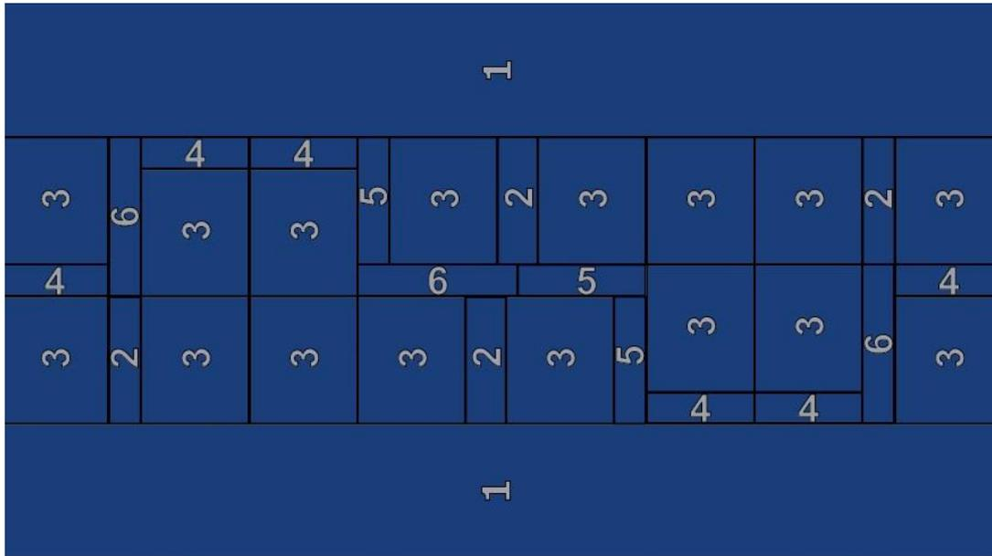
*Figure 6 - Example of the assembly of the modular block where the water and the base of the gas pipeline will be. Pieces numbered 1, 2 and 3 have a height of 10cm and pieces numbered 4, 5 and 6 have a height of 15cm.*
