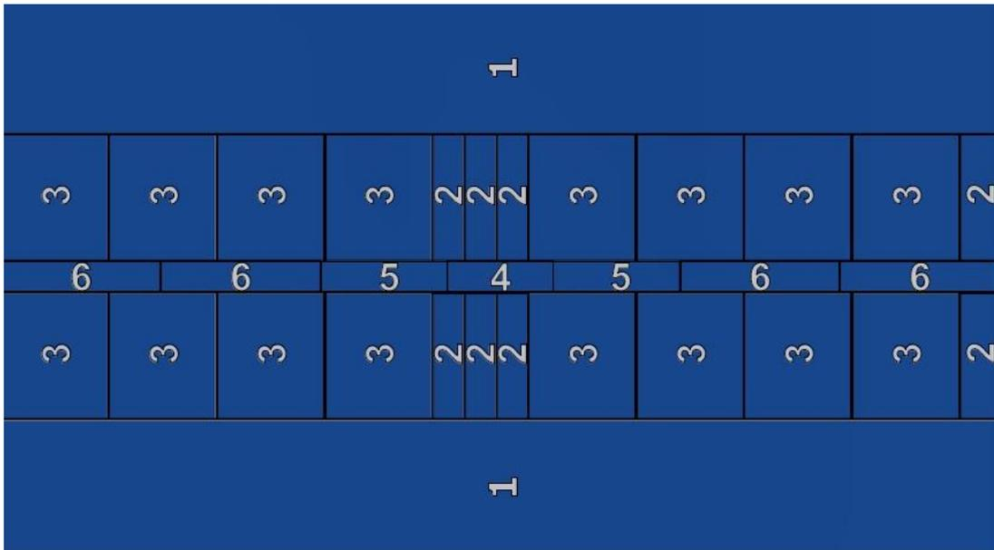
*Figure 7 - Another example of assembling the modular block where the water and the base of the gas pipeline will be.*
