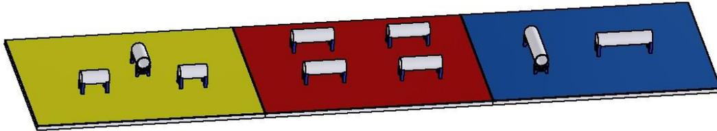
Figure 2 - Tube Collection Area - Colored bases identify the dimensions of the tubes, where the tubes are randomly arranged.
