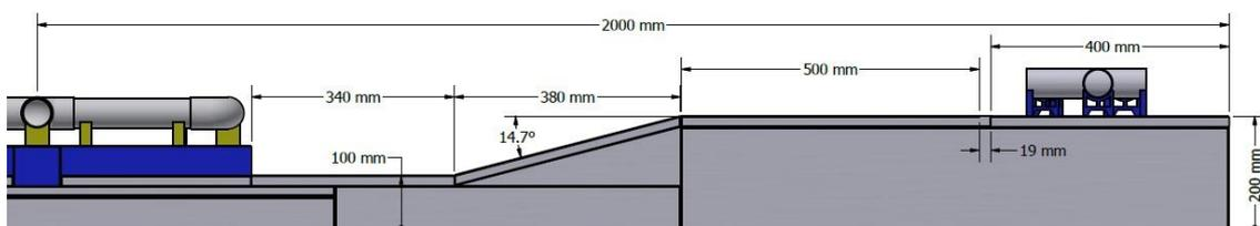
Figure 4 - Front view of half of the arena with its dimensions.
