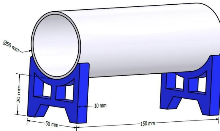
*Figure 1 - Illustration of an example of a 15cm long tube. Tube and support colors are irrelevant. The two supports must be 3cm from the end of the tube in relation to the floor and glued.*
