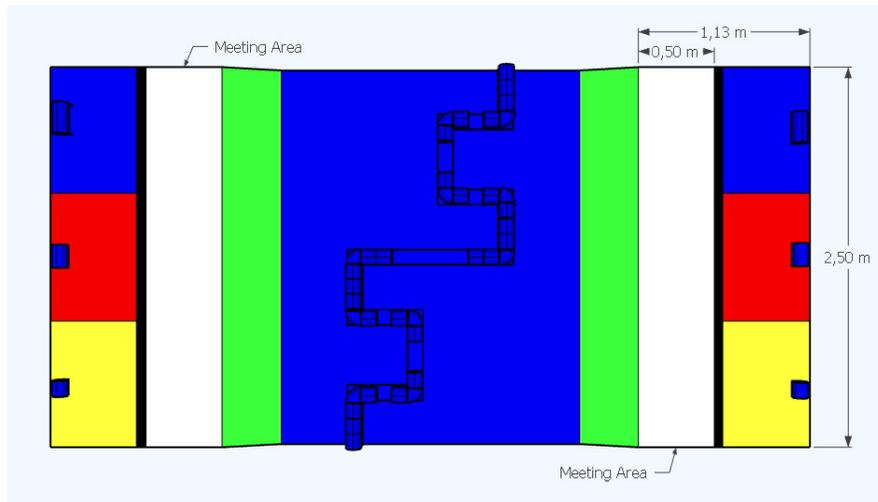
Figure 4: Top view of an arena example with its dimensions. The pipeline is merely illustrative and its layout is detailed in the next section.
