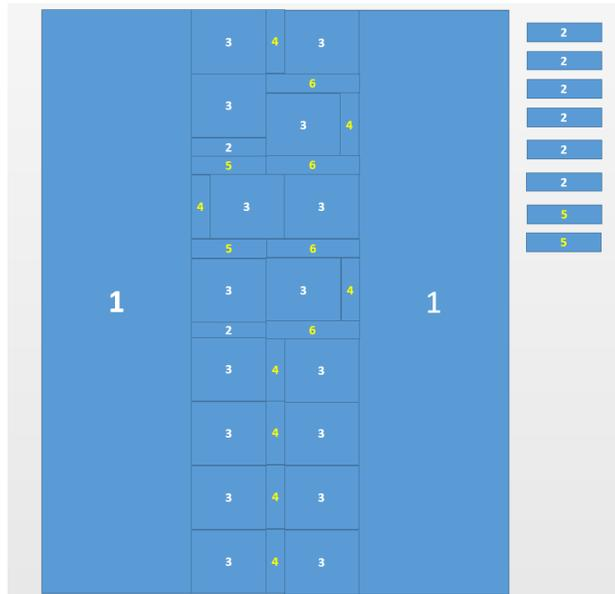
Figure 6: Example of modular block assembly with the water and the pipeline support. The numbering represents the size of the blocks and the color of the numbers are their height, white numbers are blocks of  $0.1m$  and yellow numbers are blocks of  $0.15m$ . The remaining blocks in this assembly are on the right.
