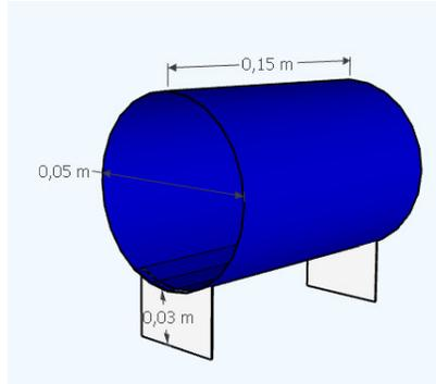
Figure 2: Example of 15cm long pipe. The colors of the pipes and the stands are irrelevant. The two MDF/MDP stands should be 3cm from the end of the pipe to the floor and glued.
