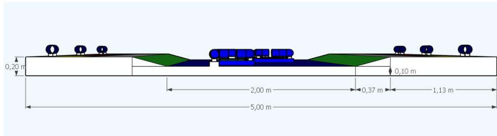
Figure 3: Front view of an arena example with its dimensions.
