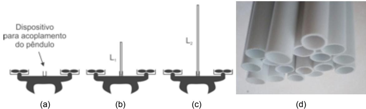
Figure 1. Positioning of the inverted pendulum to the challenge of stability and balance: a) flying robot with the device for coupling the inverted pendulum; b) flying robot with inverted pendulum  $L_1$  size; c) flying robot with inverted pendulum  $L_2$  size; d) pendulum examples.
