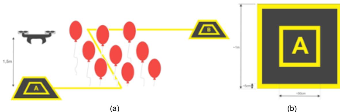
Figure 2. Illustration of trajectory tracking with obstacle avoidance challenge: a) the flying robot should move from "A" to "B" position in a place with balloons; b) approximate dimensions of the landing and takeoff areas.
