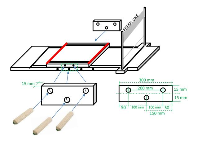
2 (two) pieces of wood (MDF) with height equal of two thickness of MDF with 3 holes must be used to lock the square piece with arena in four position.
