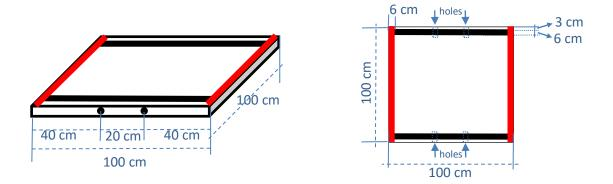
This extra piece of wood in square form will be used as an obstacle over the running arena in the extra challenge. The piece can be positioned on the arena like the figure below:
