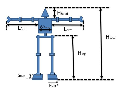
Figure 1 – Measuments of the humanoid robot for IEEE HRR competition
