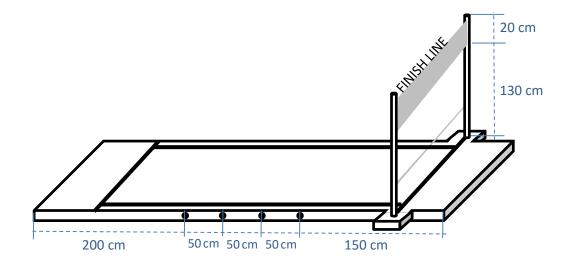
The rectangular MDF must have 4 holes for wooden dowel of 3,5mm of diameter on both sides. Wooden dowel is also called *cavilha* in Portuguese language and *perno de madera* in Spanish.
